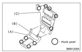
3) Remove fitting screws, and slightly pull radio out from center console.
