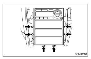
4) Disconnect electric connectors and antenna feeder cord and then disconnect heater control unit.
