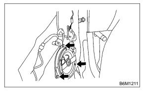
3) Disconnect harness connector and remove front speaker.
