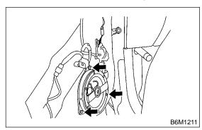
3) Disconnect harness connector and remove rear speaker.
