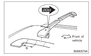
4) Tighten end support and lower clamp using TORX  $^{\!\!\!\!\!^{\otimes}}$  bolt T30.
