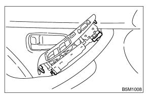
4) Remove three screws and clips.
