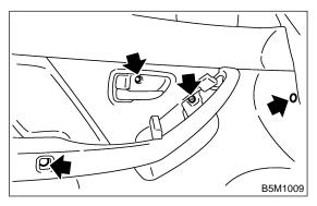
5) Remove gusset cover. Disconnect electrical connectors to remove speaker.
