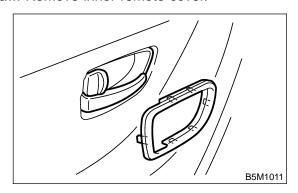
2) Remove two hooks of switch panel to remove power window main switch.
