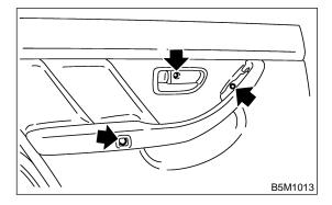
4) Remove seven clips of trim panel using clip remover to remove trim panel.
