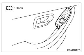
3) Remove three screws and clips.
