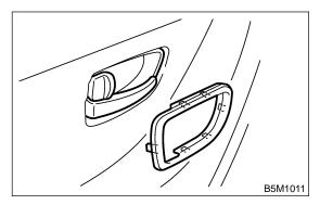
2) Remove two hooks of switch panel to remove power window sub switch and disconnect electrical connector.
