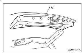
2) Remove caps and screws, and then detach high-mounted stop light cover (A).
