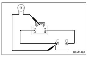
Connect battery and turn signal light bulb to the module, as shown in the figure. The module is properly functioning if it blinks when power is supplied to the circuit.
