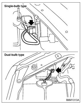
3) Remove three bolts and disconnect connectors, and then detach headlight assembly.
