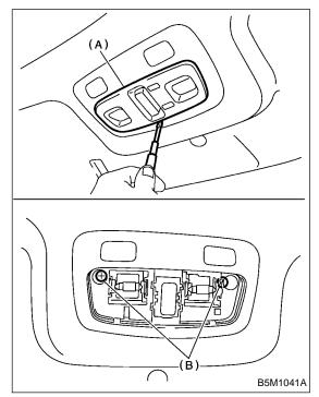
2) Disconnect harness connectors and remove spot light.
