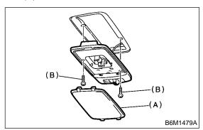
2) Disconnect harness connectors and remove the light.
