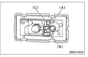
Turn the switch each position and check continuity between terminals.
