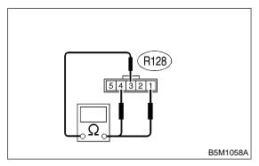
Check continuity between terminals when operating the switch.
