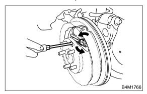
• If brake drum is difficult to remove, drive it out by installing an 8-mm bolt into bolt hole in brake drum.
