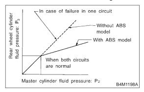
4) For the oil pressure in case of split point, refer to "SPECIFICATIONS".
