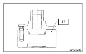
2) Using ST1, ST2 and ST3, press hub unit bearing into hub.
