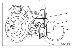
8) Remove disc rotor from hub.
