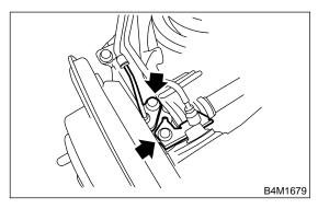
7) Remove brake caliper from back plate and suspend it from stabilizer using a piece of wire.
