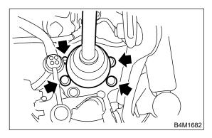
10) Remove hub unit bearing.
