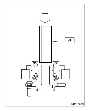
2) Using ST and a puller (common hand tool), remove bearing inner race.
