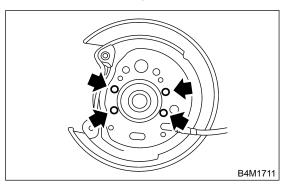
2) Tighten four bolts to back plate.
