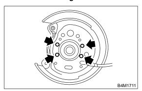
Tighten four bolts to back plate.
