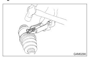
17) Cut off band with an allowance of about 10 mm (0.39 in) left from the clip and bend this allowance over the clip.
