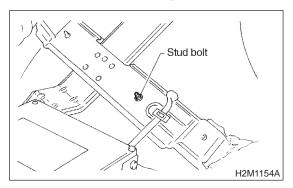
9) Use engine grounding terminal or engine proper as the grounding point to the body when measuring voltage and resistance in the engine compartment.
