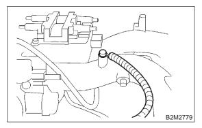
10) Use TCM mounting stud bolts at the body head grounding point when measuring voltage and resistance inside the passenger compartment.
