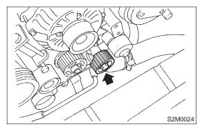
6) Install automatic belt tension adjuster which tension rod is holded with pin. <Ref. to ME(H4)-47 AUTOMATIC BELT TENSION ADJUSTER ASSEMBLY AND BELT IDLER, INSTALLATION, Timing Belt Assembly.>
