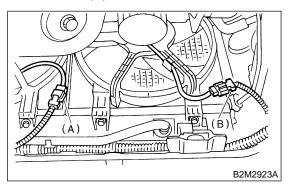
6) Disconnect radiator outlet hose and heater hose from water pump.
