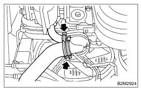
15) Connect connectors to radiator main fan (A) and sub fan (B) motors.
