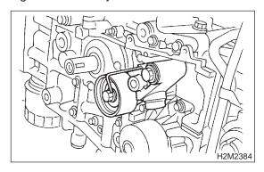
7) Install timing belt. <Ref. to ME(H4)-48 TIMING BELT, INSTALLATION, Timing Belt Assembly.>
