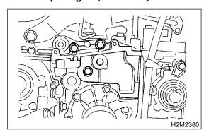
4) Install left-hand camshaft sprockets by using ST.
