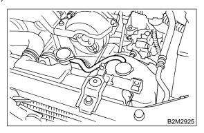
12) Install air intake duct.
