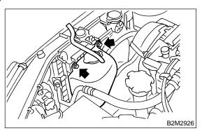
11) Remove radiator main fan and sub fan assemblies. <Ref. to CO(H4)-20 REMOVAL, Radiator Main Fan and Fan Motor.> and <Ref. to CO(H4)-23 REMOVAL, Radiator Sub Fan and Fan Motor.>
