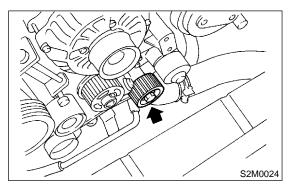
16) Remove left-hand camshaft sprocket by using
