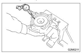
4) Check clearance between impeller and pump case
