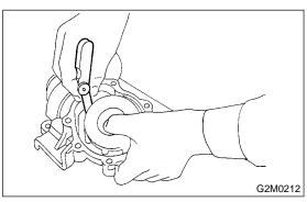
5) After water pump installation, check pulley shaft for engine coolant leaks. If leaks are noted, replace water pump assembly.
