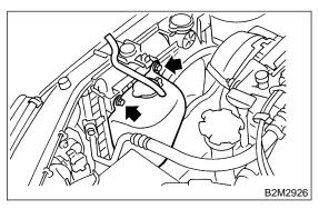
7) Install air intake duct.
