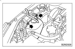
12) Disconnect radiator inlet hose from engine.
