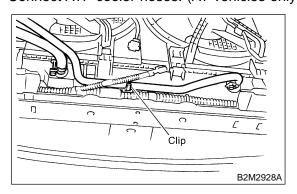
10) Connect connectors to radiator main fan motor and sub fan motor.
