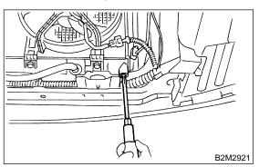
5) Disconnect connectors of radiator main fan (A) and sub fan (B) motor.
