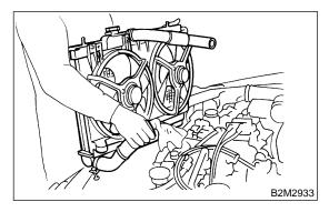
3) Install radiator brackets and tighten bolts.
