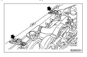
14) Detach power steering hose from the clip on the radiator.
