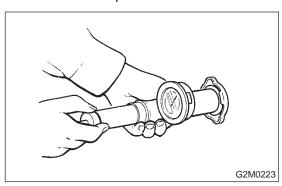
2) Increase pressure until tester gauge pointer stops. Radiator cap is functioning properly if it holds the service limit pressure for five to six seconds.
