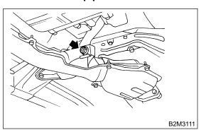
10) Separate front catalytic converter from front exhaust pipe.
