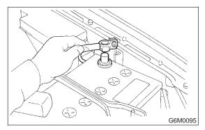
3) Disconnect front oxygen (A/F) sensor connector.
