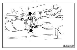
8) Remove bolts which hold front exhaust pipe onto cylinder heads.
