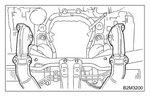
9) Remove front exhaust pipe and center exhaust pipe from hanger bracket.
