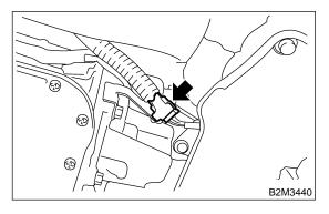
7) Separate center exhaust pipe from rear exhaust pipe.
