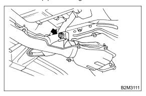
3) Tighten bolts which hold front exhaust pipe onto cylinder heads.
