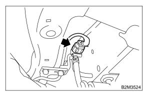
6) Disconnect pressure hose from fuel tank pressure sensor.
