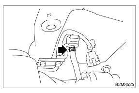
7) Remove fuel tank pressure sensor.
