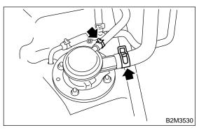
3) Remove nuts which install vent valve on fuel tank.
