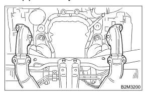
8) Remove bolt which installs front and center exhaust pipe assembly to hanger bracket.
