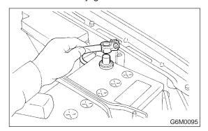
2) Disconnect front oxygen (A/F) sensor connector.
