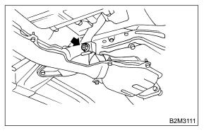
8) Connect rear oxygen sensor connector.
