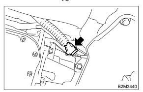
5) Separate front and center exhaust pipe assembly from rear exhaust pipe.
