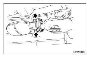
2) Separate rear exhaust pipe from muffler.
