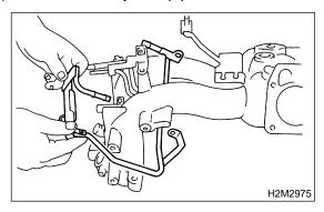
29) Remove bolt which installs fuel pipes on intake manifold.
