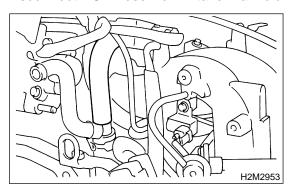
10) Disconnect engine coolant hose from throttle body.
