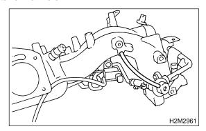
19) Install air assist injector solenoid valve to bracket.
