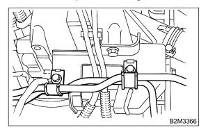
(5) Remove bolts which install power steering pump bracket.
