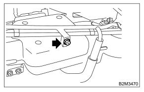
25) Remove fuel pipe assembly and pressure regulator, from intake manifold.
