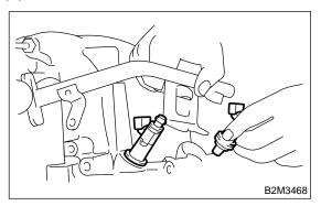
20) Disconnect air by-pass hoses from intake manifold.
