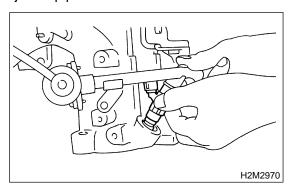
25) Disconnect air by-pass hoses from intake manifold.
