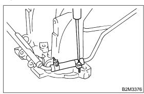
4) Install fuel injector pipe.
