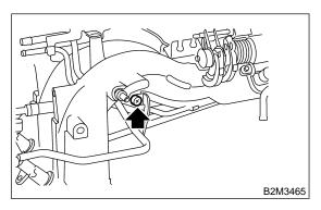
18) Remove two bolts which hold fuel pipes on the left side of intake manifold.
