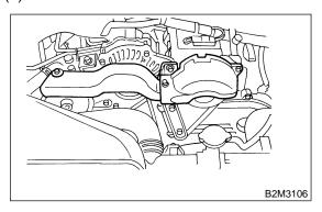
(3) Loosen lock bolt and slider bolt, and remove power steering pump drive V-belt.
