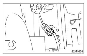
15) Disconnect connector from crankshaft position sensor.
