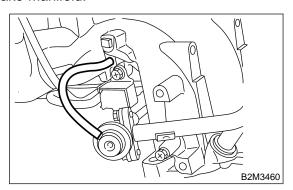
19) Install throttle body to intake manifold.
