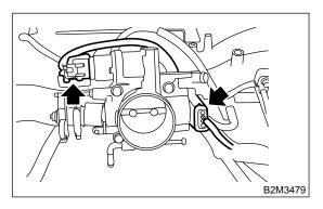
7) Disconnect air by-pass hose from throttle body.
