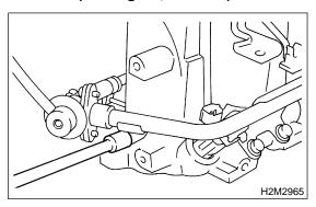
9) Tighten two bolts which install fuel pipes on the left side of intake manifold.
