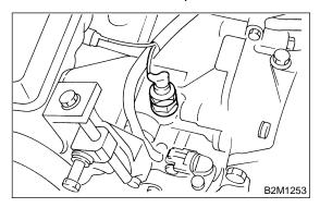
5) Connect connector to crankshaft position sensor.
