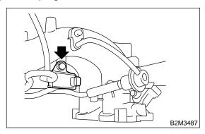
12) Connect hoses to purge control solenoid valve.
