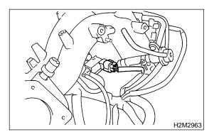
13) Remove harness bands (\*) which hold engine harness onto intake manifold.
