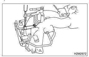
22) Loosen clamp which holds front right side fuel hose to injector pipe and remove the pipe from clamp.
