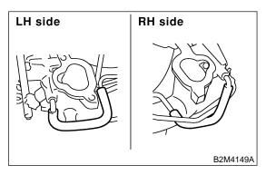
26) Loosen clamp which holds front left side fuel hose to injector pipe and remove the pipe from clamp.
