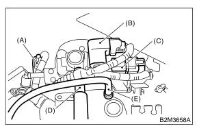
23) Install ignition coil and ignitor assembly.
