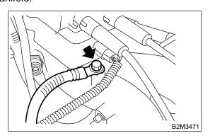
2) Disconnect connector from ignition coil and ignitor assembly.
