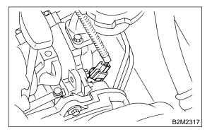
4) Connect connector to oil pressure switch.
