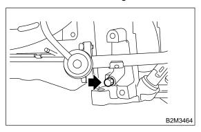
17) Remove bolt which installs injector pipe on intake manifold.
