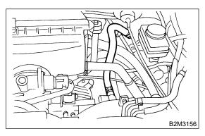
10) Connect engine coolant hose to throttle body.
