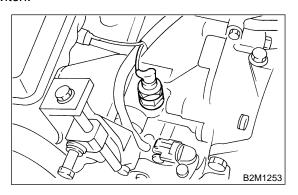
17) Disconnect connector from camshaft position sensor.
