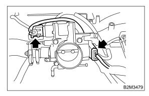
24) Connect air by-pass hose to throttle body.
