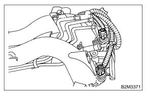
12) Disconnect connector from purge control solenoid valve.
