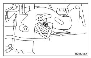
11) Install purge control solenoid valve.
