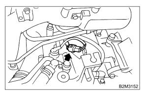
(3) Tighten bolts which install power steering pump on bracket.
