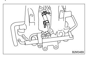
27) Loosen clamp which holds front right side fuel hose to injector pipe and remove the pipe from clamp.
