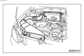
17) Connect connector to fuel pump relay.
