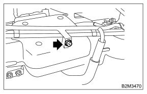
3) Connect right side fuel hose to injector pipe, and tighten clamp screw.
