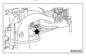
11) Install purge control solenoid valve.
