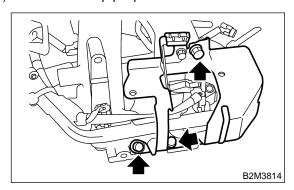
11) Disconnect connectors from fuel injectors.
