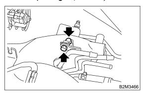
10) Tighten bolt which install injector pipe on intake manifold.
