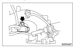
21) Remove bolt which installs injector pipe on intake manifold as shown in figure.
