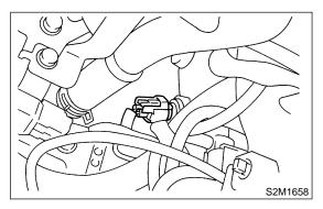
8) Install air cleaner case stay RH and engine harness bracket, and connect engine harness connectors to bulkhead connectors.
