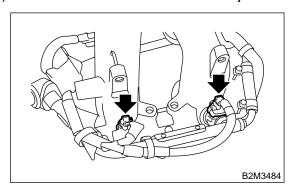
16) Disconnect connector from purge control solenoid valve.
