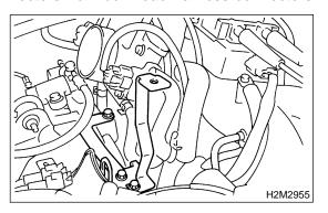
13) Disconnect connectors from engine coolant temperature sensor.
