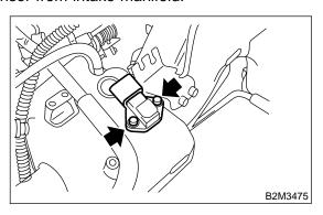
6) Disconnect connectors from throttle position sensor and idle air control solenoid valve.
