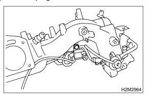
16) Remove bolt which installs injector pipe on intake manifold as shown in figure.
