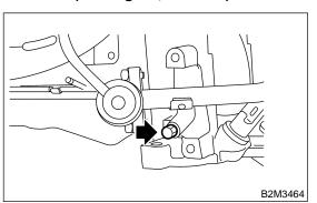
9) Tighten two bolts which install fuel pipes on the left side of intake manifold.
