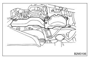
(8) Install resonator chamber.
