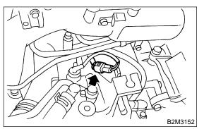
(7) Remove power steering tank from the bracket by pulling it upwards.
