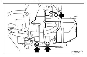
15) Disconnect connectors from fuel injectors.
