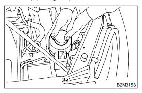
(8) Place power steering pump and tank on the right side wheel apron.
