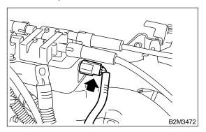
3) Remove ignition coil and ignitor assembly.
