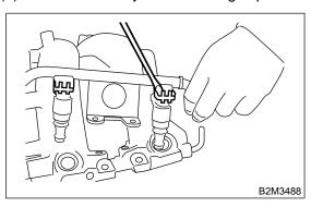
(2) Remove fuel injector while lifting up fuel injector pipe.
