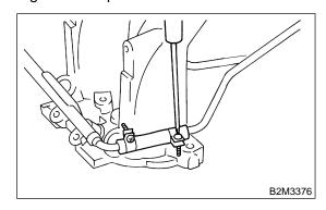
4) Install fuel injector pipe.
