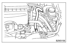
12) Remove air cleaner case stay RH and engine harness bracket, and disconnect engine harness connectors from bulkhead harness connectors.
