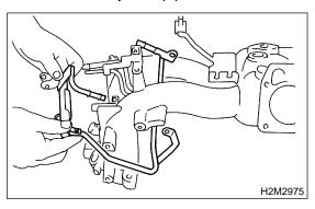
24) Remove bolt which installs fuel pipes on intake manifold.
