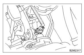
18) Disconnect fuel hoses from fuel pipes.
