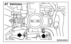
11) Connect PCV hose to intake manifold.
