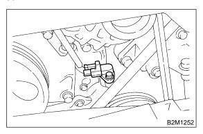
16) Disconnect connector from oil pressure switch.
