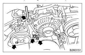
(4) Install power steering pipes onto right side intake manifold protector.
