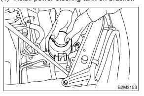
(2) Connect connector to power steering pump switch.
