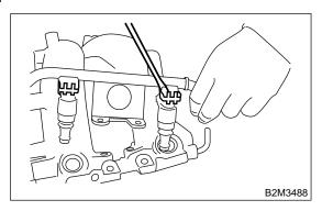
8) Tighten bolt which installs injector pipe on intake manifold.
