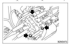
4) Disconnect connector from intake air temperature and pressure sensor.
