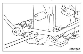
22) Remove bolt which installs injector pipe on intake manifold.
