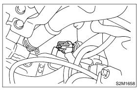
4) Remove engine coolant temperature sensor.
