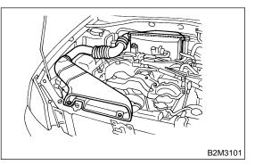
3) Disconnect connector from engine coolant temperature sensor.
