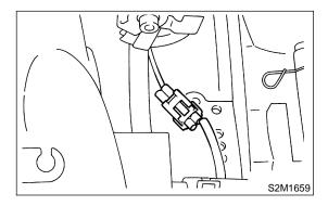
4) Remove knock sensor from cylinder block.
