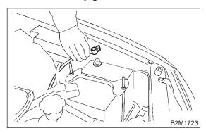
2) Remove idle air control solenoid valve. <Ref. to FU(H4)-53 MT VEHICLES, REMOVAL, Idle Air Control Solenoid Valve.>
