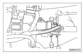
4) Remove intake manifold pressure sensor from throttle body.
