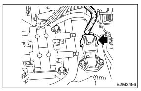
4) Remove intake air temperature and pressure sensor.
