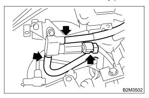
3) Remove air assist injector solenoid valve from intake manifold.
