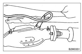
3) Connect connector to rear oxygen sensor.
