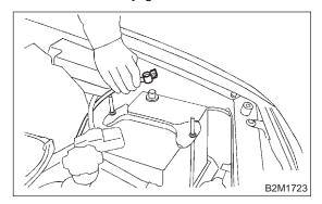
2) Disconnect connector from rear oxygen sensor.
