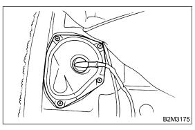
9) Disconnect connector from fuel sub level sensor.
