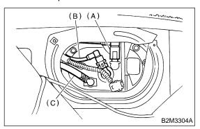
13) Remove nuts which install fuel pump assembly onto fuel tank.
