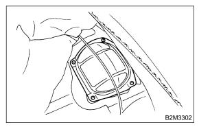
10) Disconnect connector from fuel pump.
