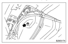
7) Tighten fuel drain plug and install front right side fuel tank cover.
