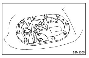
14) Take off fuel pump assembly from fuel tank.
