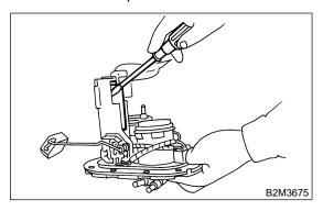
2) Disconnect connector from fuel pump.
