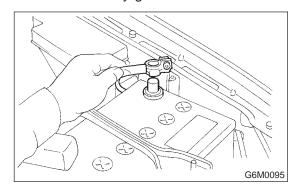
2) Disconnect connector from intake air temperature sensor. (MT vehicles)
