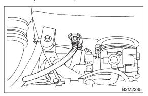
3) Loosen clamp which connects air cleaner case to throttle body.
