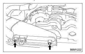
2) Remove bolt which installs air intake duct on body.
