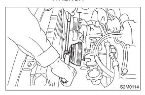
11) Remove water pump. <Ref. to CO(H4)-8 REMOVAL, Water Pump.>
