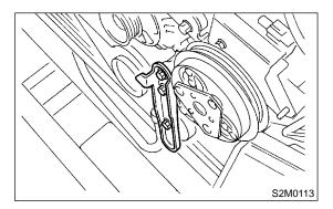
10) Remove crankshaft pulley by using ST. ST 499977100 CRANKSHAFT PULLEY WRENCH
