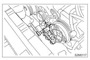
15) Remove oil pump by using flat bladed screw-driver.
