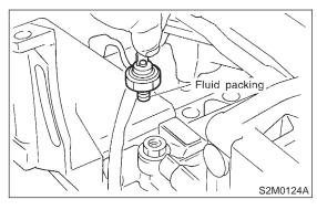
2) Install oil pressure switch onto engine block.
