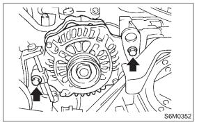
5) Install front side V-belt and adjust it.<Ref. to ME(H4)-43 INSTALLATION, V-belt.>6) Install V-belt cover.
