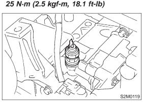
3) Connect terminal of oil pressure switch.
