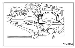
7) Connect connector and terminal to generator.
