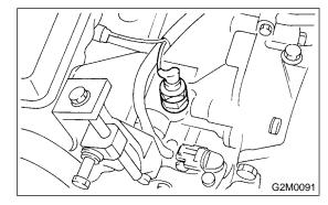
3) Remove oil pressure switch.
