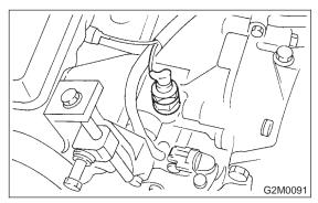
4) Install generator on bracket and temporarily tighten installing bolts.
