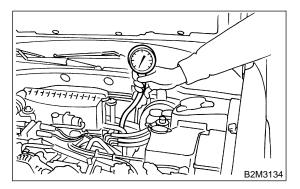
Vacuum pressure (at idling, A/C "OFF"): Less than -60.0 kPa (-450 mmHg, -17.72 inHg)
