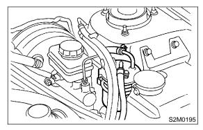
4) Connect connector of fuel pump relay.
