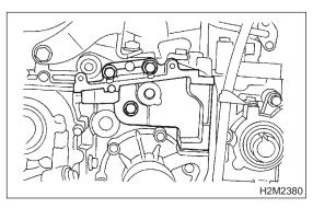
10) Remove camshaft position sensor support. (LH side only)
