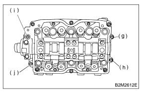
(3) Install valve rocker assembly.
