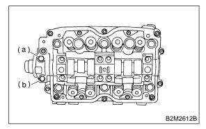
(2) Equally loosen bolts (c) through (j) all the way in alphabetical sequence.
