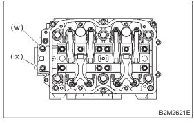
3) Apply a coat of grease to oil seal lips and install oil seal (A) on camshaft using ST1 and ST2.
