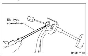
13) Disconnect accelerator cable stopper from bracket.
