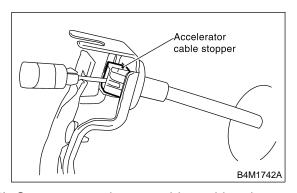
14) Separate accelerator cable and bracket.
