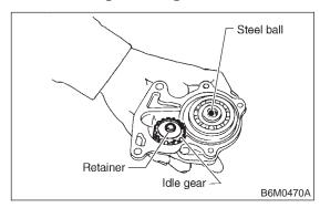
3) Installing armature to yoke
