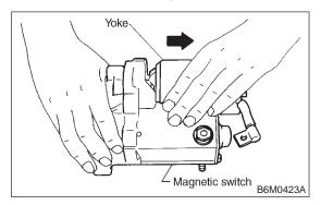
4) Remove screws securing end frame to brush holder.
