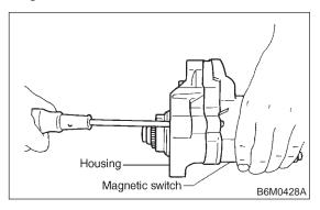
9) Remove housing from magnetic switch.
