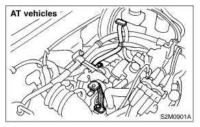
5) Disconnect connector and terminal from starter.
