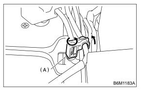
2) Disconnect the positive (+) terminal after disconnecting the negative (-) terminal of battery.
