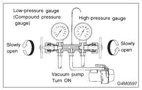
5) After the low-pressure gauge reaches 100.0 kPa (750 mmHg, 29.5 inHg) or higher, evacuate the system for approx. 15 minutes.
