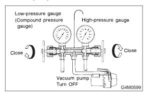
7) Note the low-pressure gauge reading.
