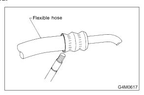
11) Disconnect the drain hose from the evaporator case, and check the hose end for at least 10 seconds
