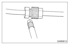
Connection between the tube and nut
