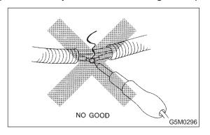
• Install the wire harness securely with the specified clips to avoid interference or tangled up with other parts.
