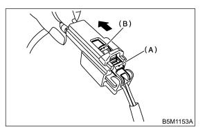
3) With slide lock (B) pulled, remove lock arm (A) to its original position, and then pull in the direction of the arrow and separate the connector.
