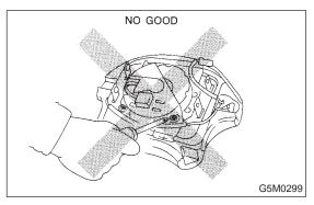
Do not check continuity of the airbag module (driver, passenger, and side) with airbag removed from the vehicle.
